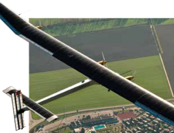
The Solar Impulse, a solar airplane fitted with 12,000 solar cells, completed a 26-hour flight in July 2010, a record flying time for a solar-powered aircraft.
